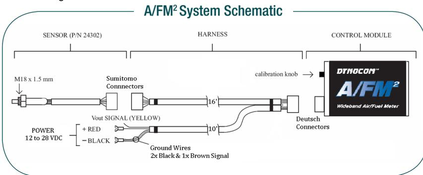
Figure 3 - A/FM<sup>2</sup> System Schematic
