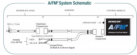
Figure 3 - A/FM<sup>2</sup> System Schematic
