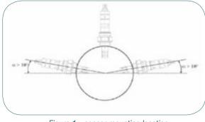
Figure 1 - sensor mounting location
