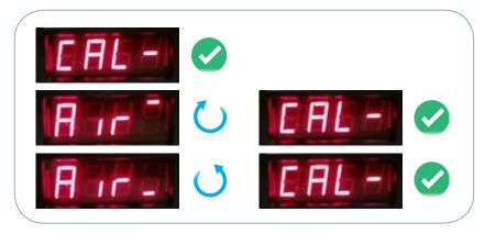
5. Disconnect the power from the harness. When the AFR sensor cools down, install it in the exhaust and do not touch the calibration knob until the next time the system needs to be calibrated or when replacing the units AFR sensor with a new one.
