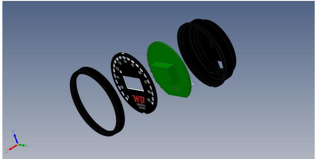
Just pop the bezel out first. Either push the faceplate out from the connector at the back or pull it out from the front side via tweezers or small screwdriver. Take the PCB board out when you need to replace it with a new one.
